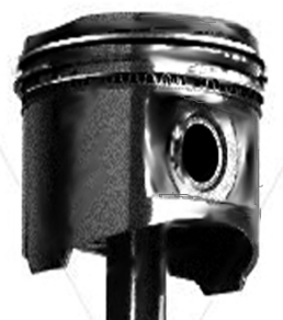
Good condition piston with UPOIL P 1000
